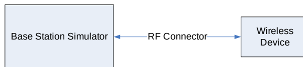
Figure 9-1 Power Measurement Setup
