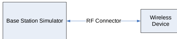
Figure 9-3 Power Measurement Setup
