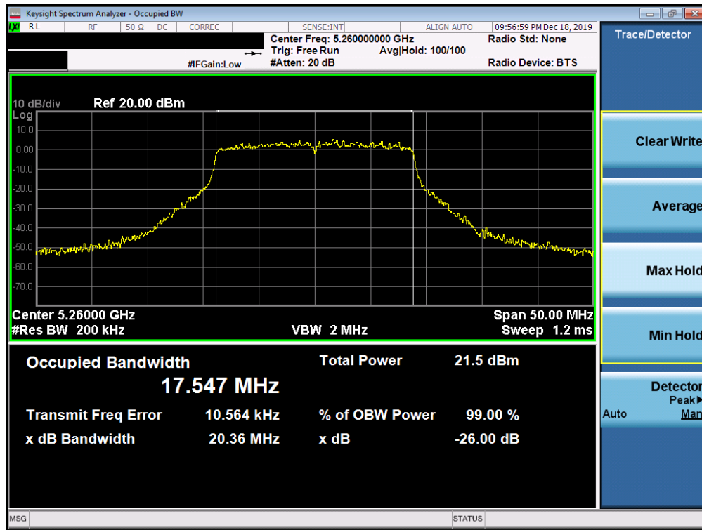
Plot 7-27. 26dB Bandwidth Plot SISO ANT1 (20MHz BW 802.11ac (UNII Band 2A) – Ch. 52)
