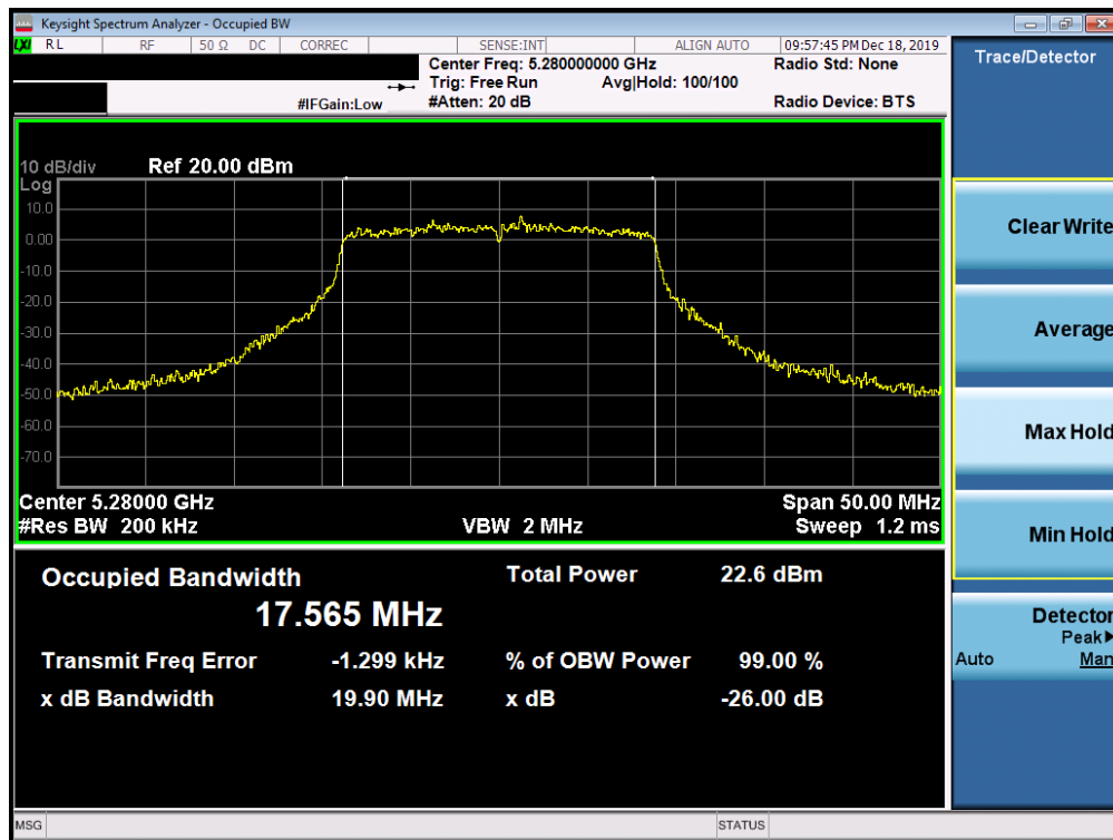
Plot 7-28. 26dB Bandwidth Plot SISO ANT1 (20MHz BW 802.11ac (UNII Band 2A) – Ch. 56)
