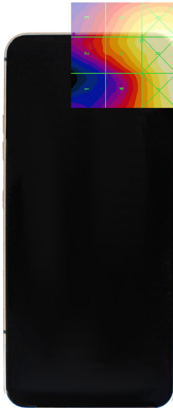
Figure 18-8 E-Field WD Scan overlay (T-Coil Centered Scan Pictured)
