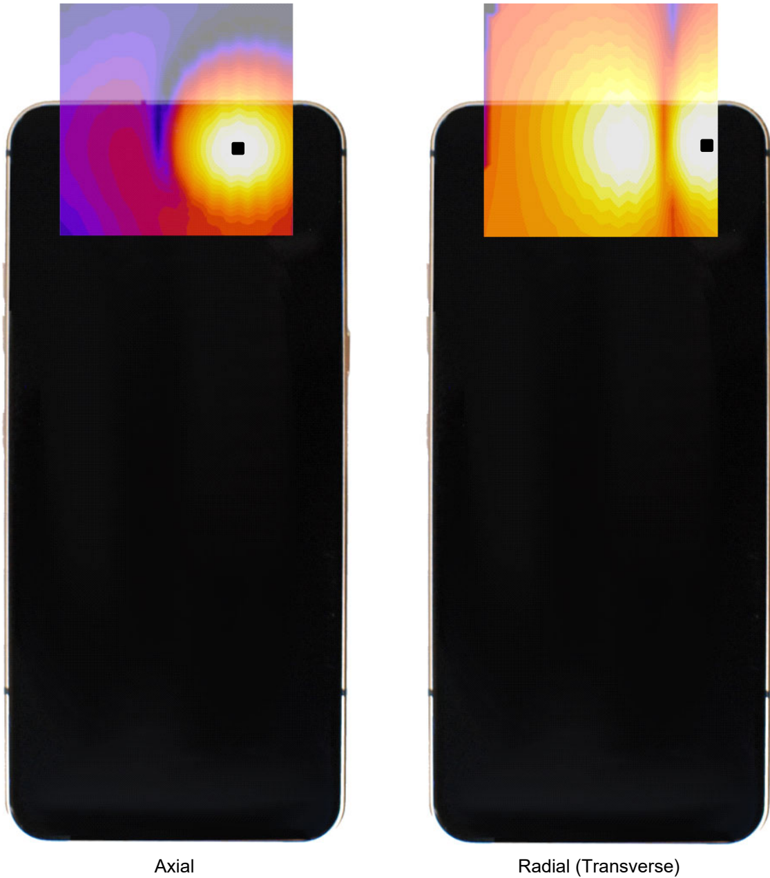
Figure 16-3 T-Coil Scan Overlay Magnetic Field Distributions
