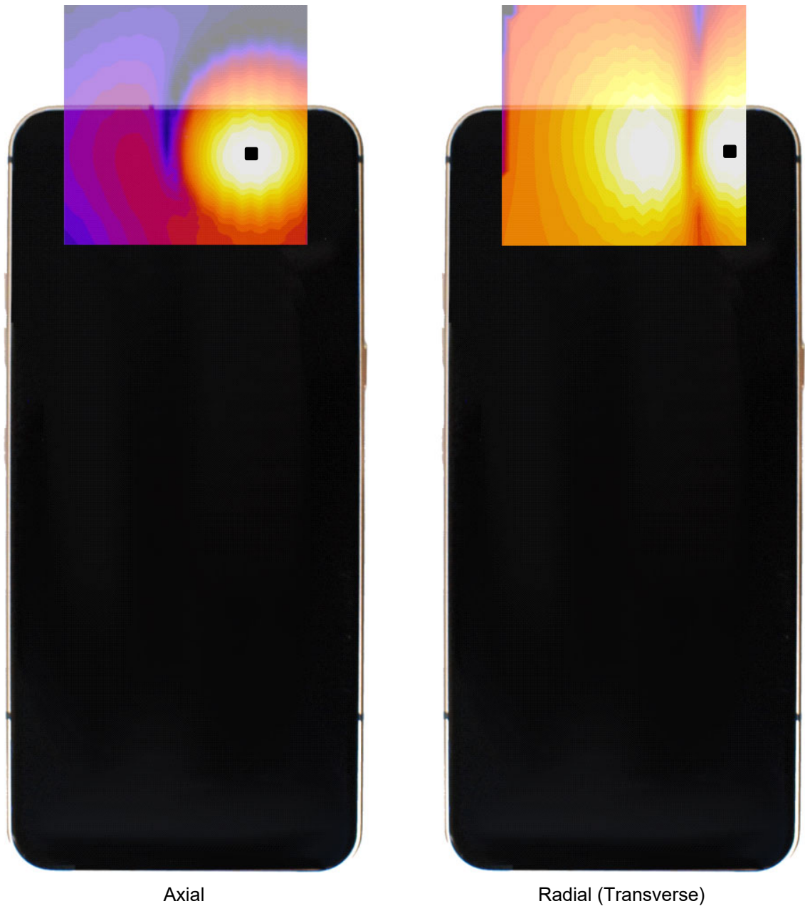
Figure 16-7 T-Coil Scan Overlay Magnetic Field Distributions
