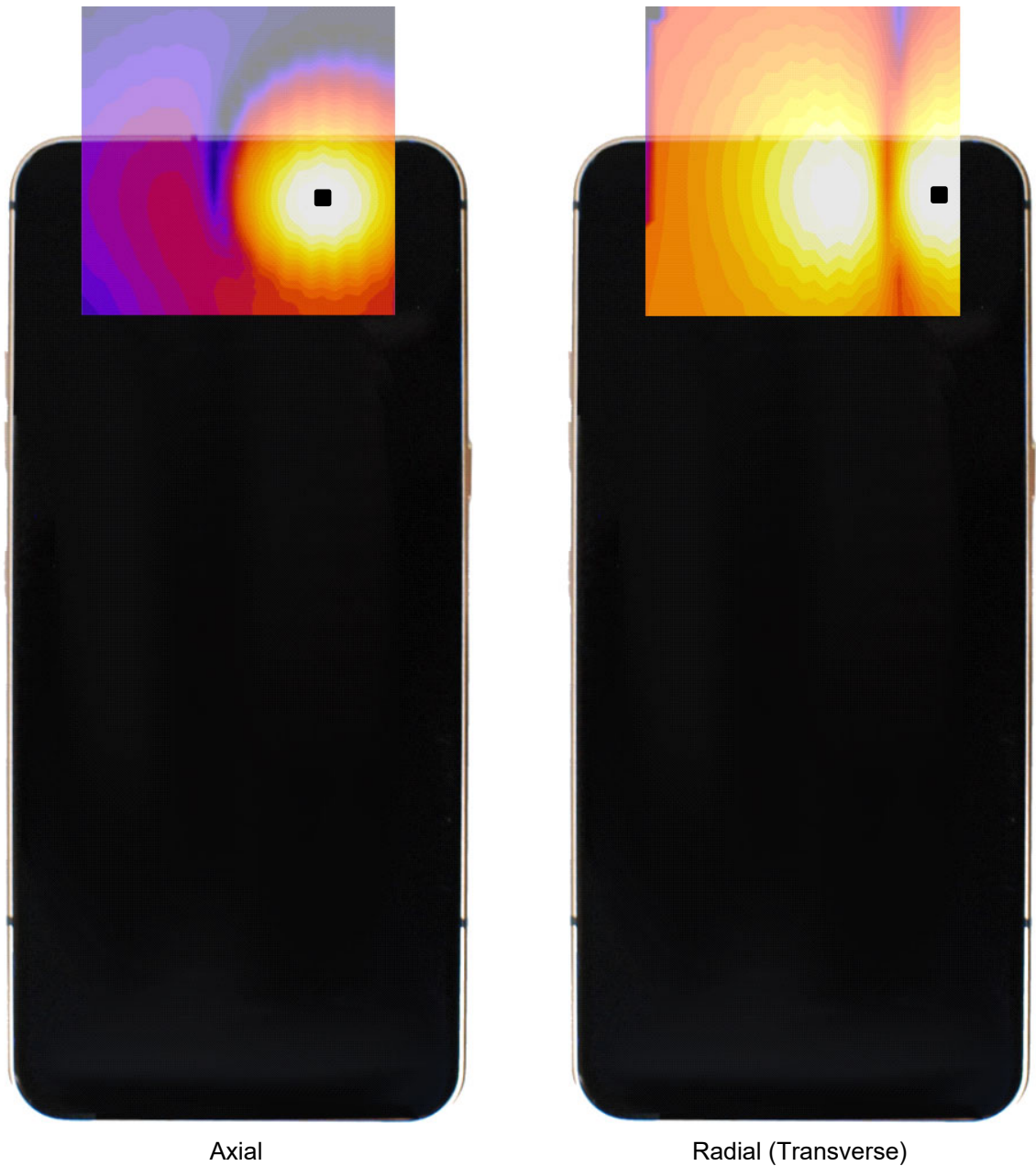
Figure 16-7 T-Coil Scan Overlay Magnetic Field Distributions
