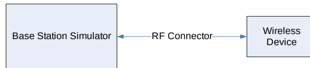
Figure 9-1 Power Measurement Setup
