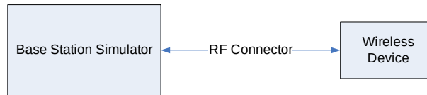
Figure 9-4 Power Measurement Setup
