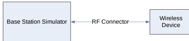
Figure 9-2 Power Measurement Setup
