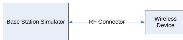
Figure 9-3 Power Measurement Setup
