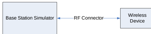
Figure 9-4 Power Measurement Setup
