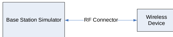
Figure 9-3 Power Measurement Setup
