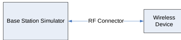
Figure 9-4 Power Measurement Setup
