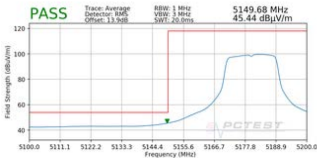
Plot 7-49. Radiated Lower Band Edge Plot SISO ANT2 (Average – UNII Band 1)
