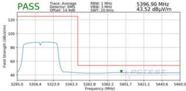
Plot 7-37. Radiated Upper Band Edge Plot SISO ANT1 (Average – UNII Band 2A)
