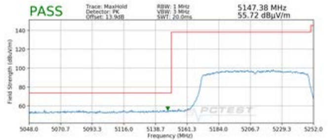
Plot 7-89. Radiated Lower Band Edge Plot MIMO (Peak – UNII Band 1)
