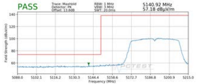
Plot 7-57. Radiated Lower Band Edge Plot SISO ANT2 (Peak - UNII Band 1)
