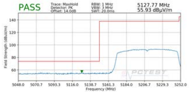
Plot 7-43. Radiated Lower Band Edge Plot SISO ANT1 (Peak – UNII Band 1)
