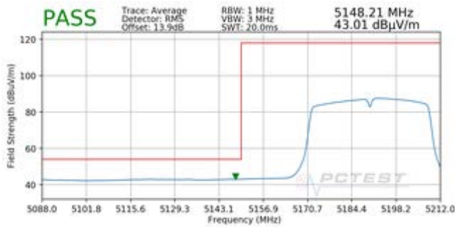
Plot 7-35. Radiated Lower Band Edge Plot SISO ANT1 (Average – UNII Band 1)
