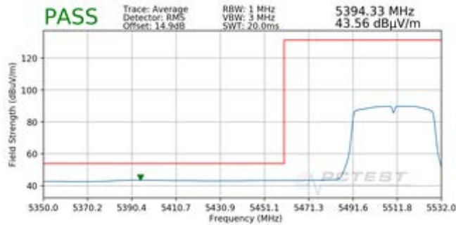
Plot 7-39. Radiated Lower Band Edge Plot SISO ANT1 (Average – UNII Band 2C)
