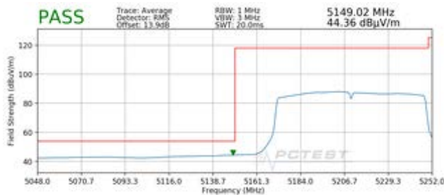
Plot 7-63. Radiated Lower Band Edge Plot SISO ANT2 (Average – UNII Band 1)
