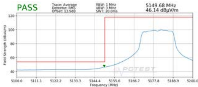
Plot 7-70. Radiated Lower Band Edge Plot MIMO (Average – UNII Band 1)
