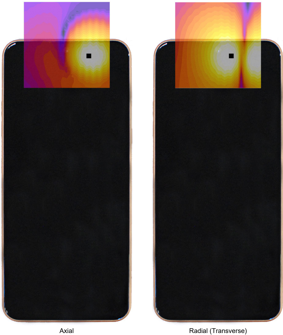
Figure 16-3 T-Coil Scan Overlay Magnetic Field Distributions
