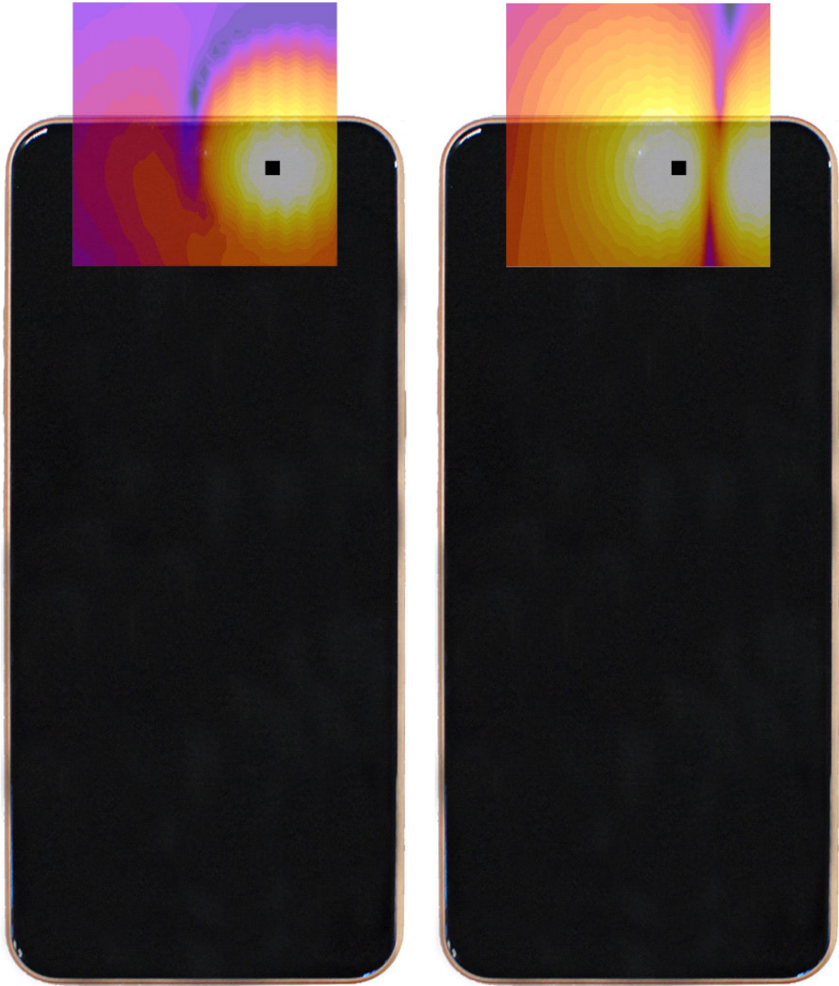
Figure 16-7 T-Coil Scan Overlay Magnetic Field Distributions
