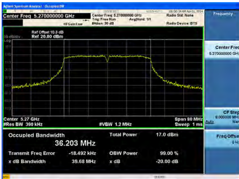
20 dB Bandwidth plot (802.11n_40 MHz BW-CH 54)
