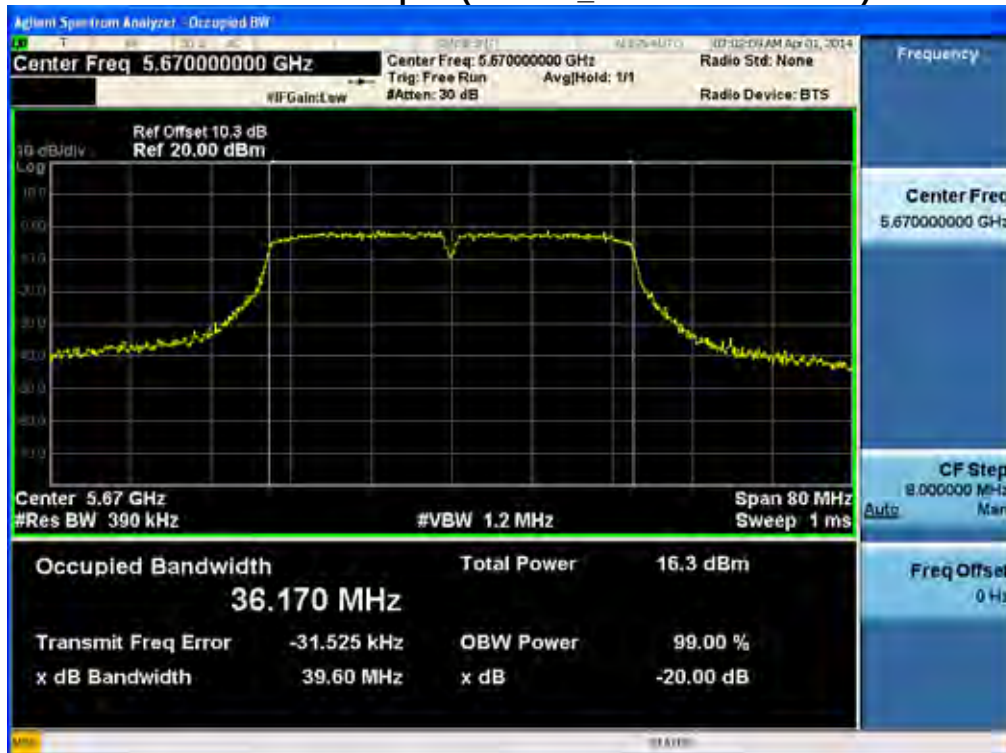
20 dB Bandwidth plot (802.11n_40 MHz BW-CH 134)
