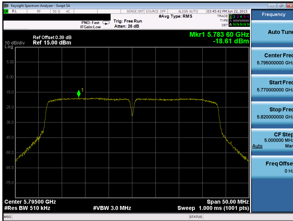
Plot 6-73. Power Spectral Density Plot (40MHz BW 802.11n (UNII Band 3) – Ch. 159)
