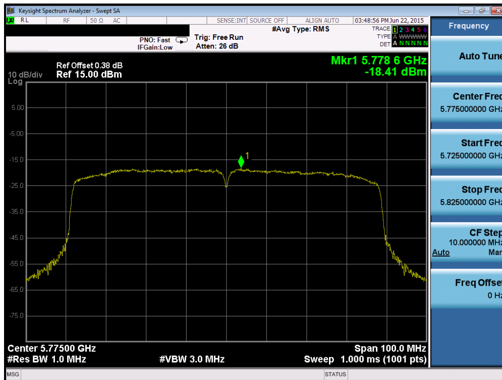
Plot 6-74. Power Spectral Density Plot (80MHz BW 802.11ac (UNII Band 3) – Ch. 155)
