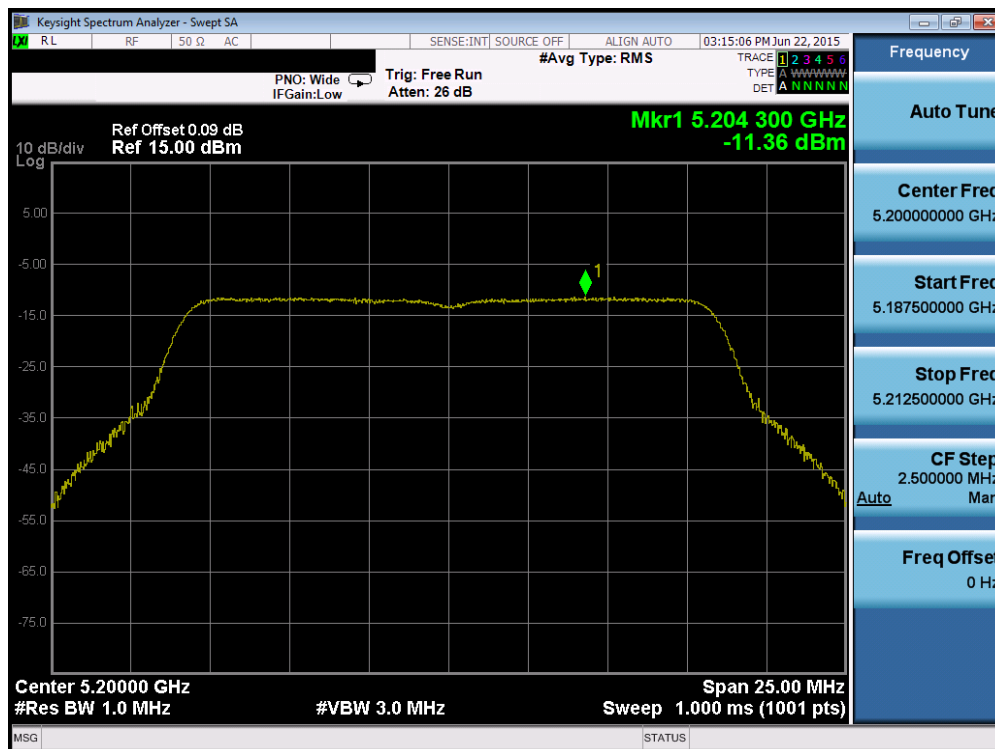
Plot 6-39. Power Spectral Density Plot (802.11a (UNII Band 1) – Ch. 40)
