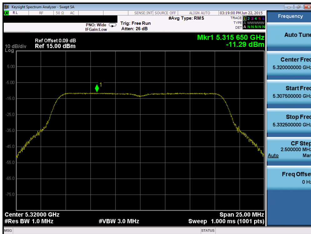
Plot 6-49. Power Spectral Density Plot (802.11a (UNII Band 2A) – Ch. 64)
