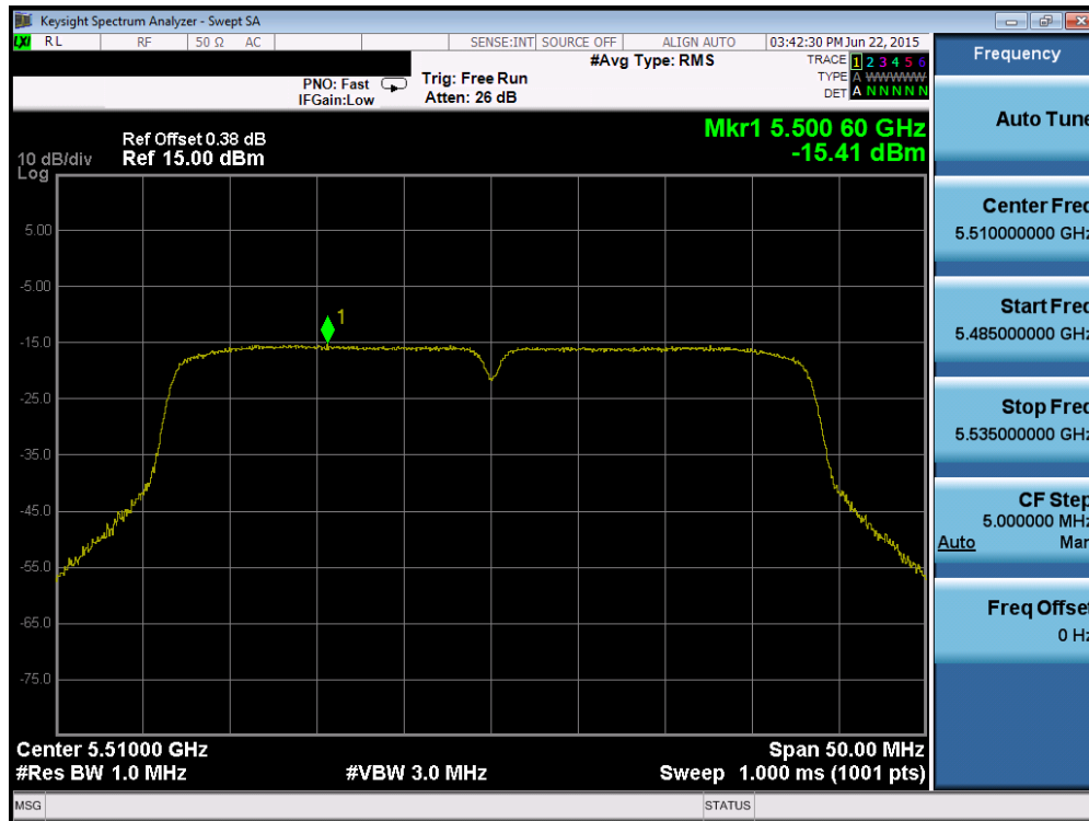
Plot 6-62. Power Spectral Density Plot (40MHz BW 802.11n (UNII Band 2C) – Ch. 102)
