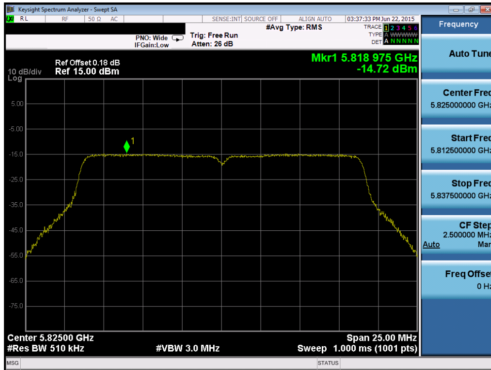
Plot 6-71. Power Spectral Density Plot (20MHz BW 802.11n (UNII Band 3) – Ch. 165)
