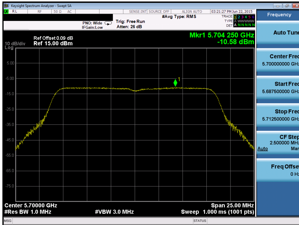
Plot 6-58. Power Spectral Density Plot (802.11a (UNII Band 2C) – Ch. 140)
