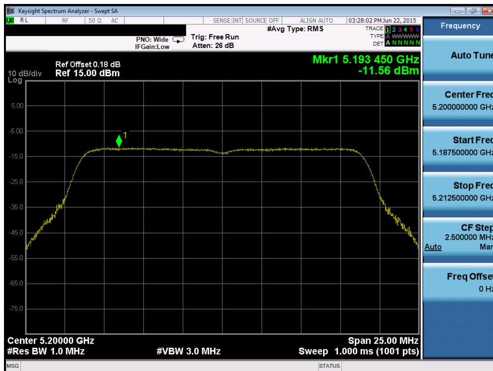
Plot 6-42. Power Spectral Density Plot (20MHz BW 802.11n (UNII Band 1) – Ch. 40)
