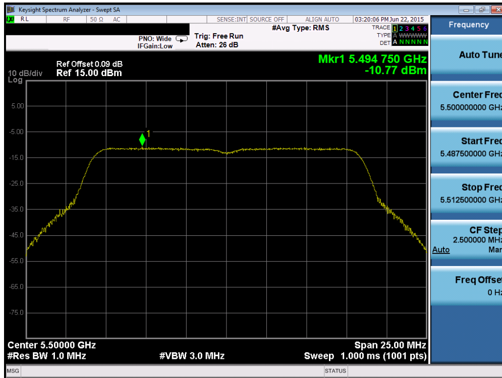
Plot 6-56. Power Spectral Density Plot (802.11a (UNII Band 2C) – Ch. 100)
