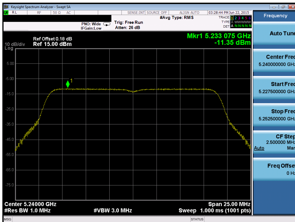
Plot 6-43. Power Spectral Density Plot (20MHz BW 802.11n (UNII Band 1) – Ch. 48)
