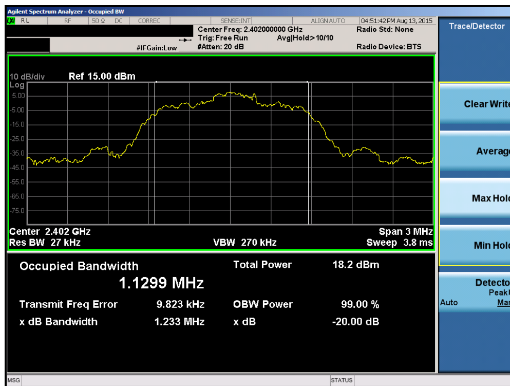
Plot 6-1. 20dB Bandwidth Plot (Bluetooth, 1Mbps – Ch. 0)
