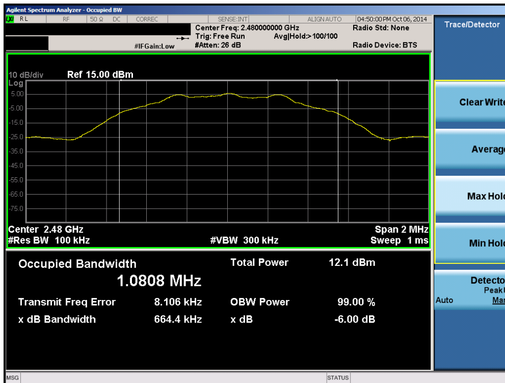
Plot 6-3. 6dB Bandwidth Plot (Bluetooth (LE) – Ch. 39)
