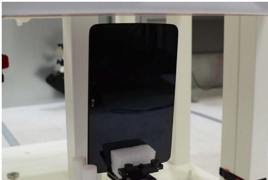
SAR Test Setup Photo 4: Top Edge at 14 mm
