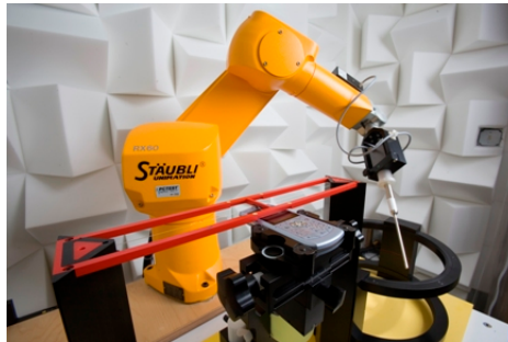
Figure 5-3 SPEAG Robotic System
