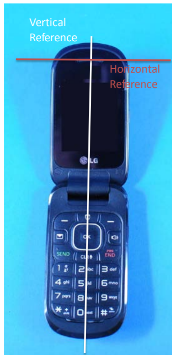
SAR Test Setup Photo 8 - Vertical and Horizontal Reference Lines
