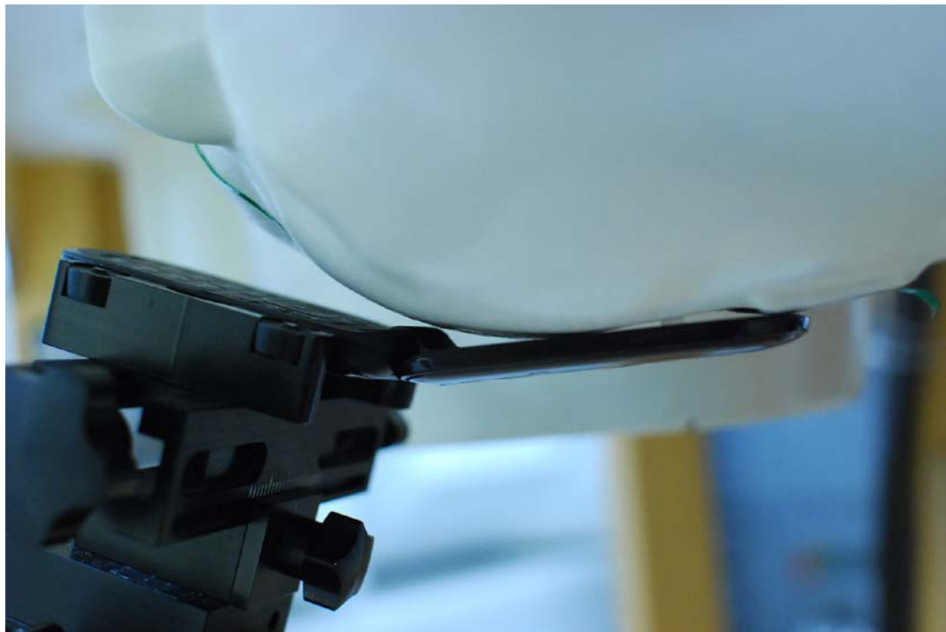
SAR Test Setup Photo 4 - Left Cheek
