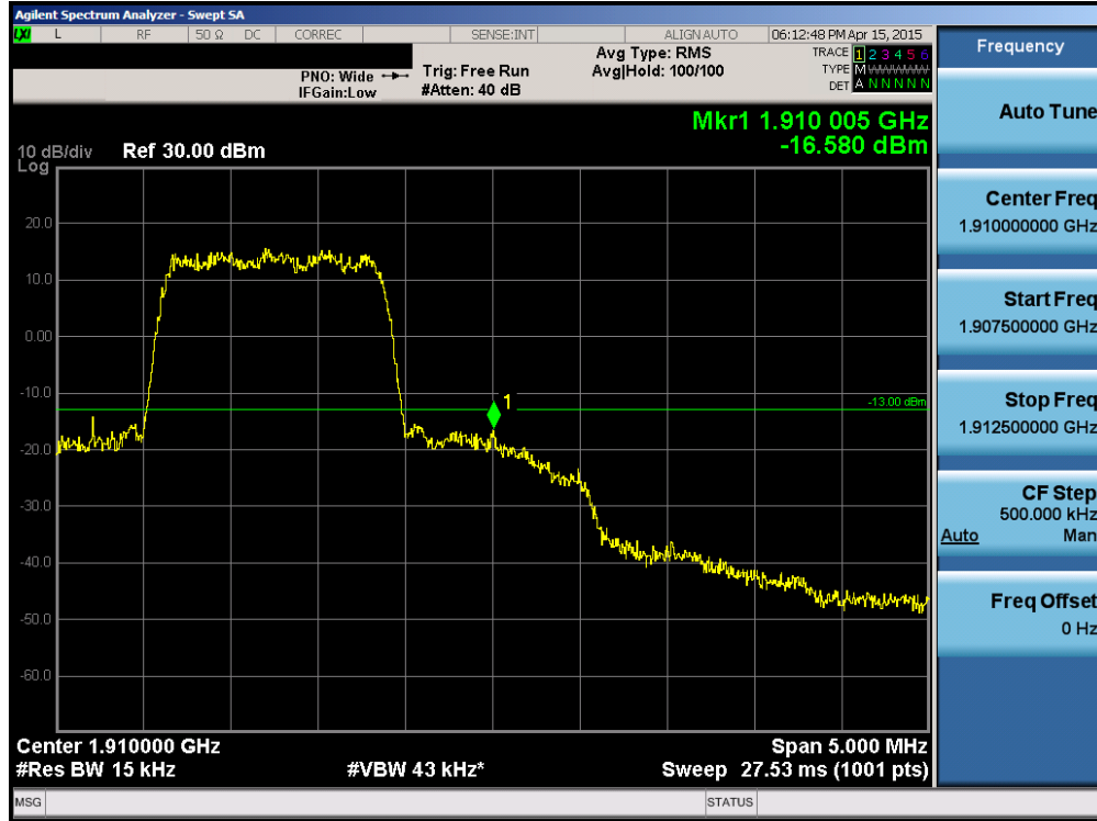
Plot 6-55. Band Edge Plot (PCS CDMA Mode – Ch. 1175)
