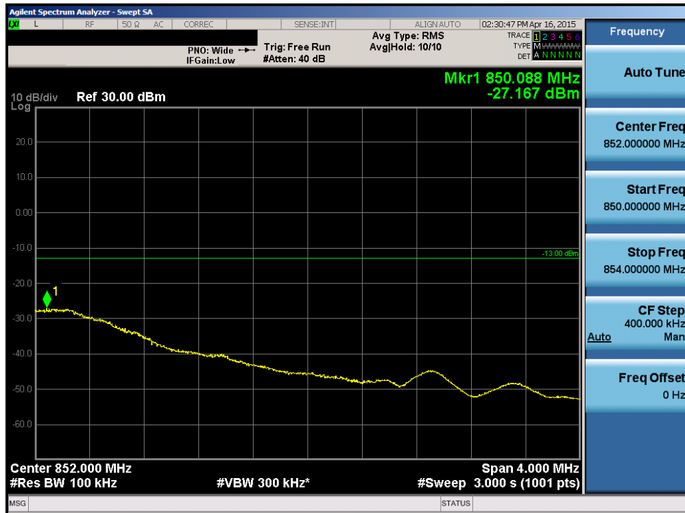
Plot 6-52. 4MHz Span Plot (Cellular CDMA Mode – Ch. 777)
