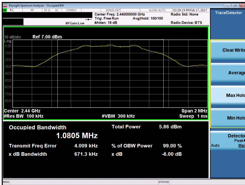
Plot 7-2. 6dB Bandwidth Plot (Bluetooth (LE) – Ch. 19)
