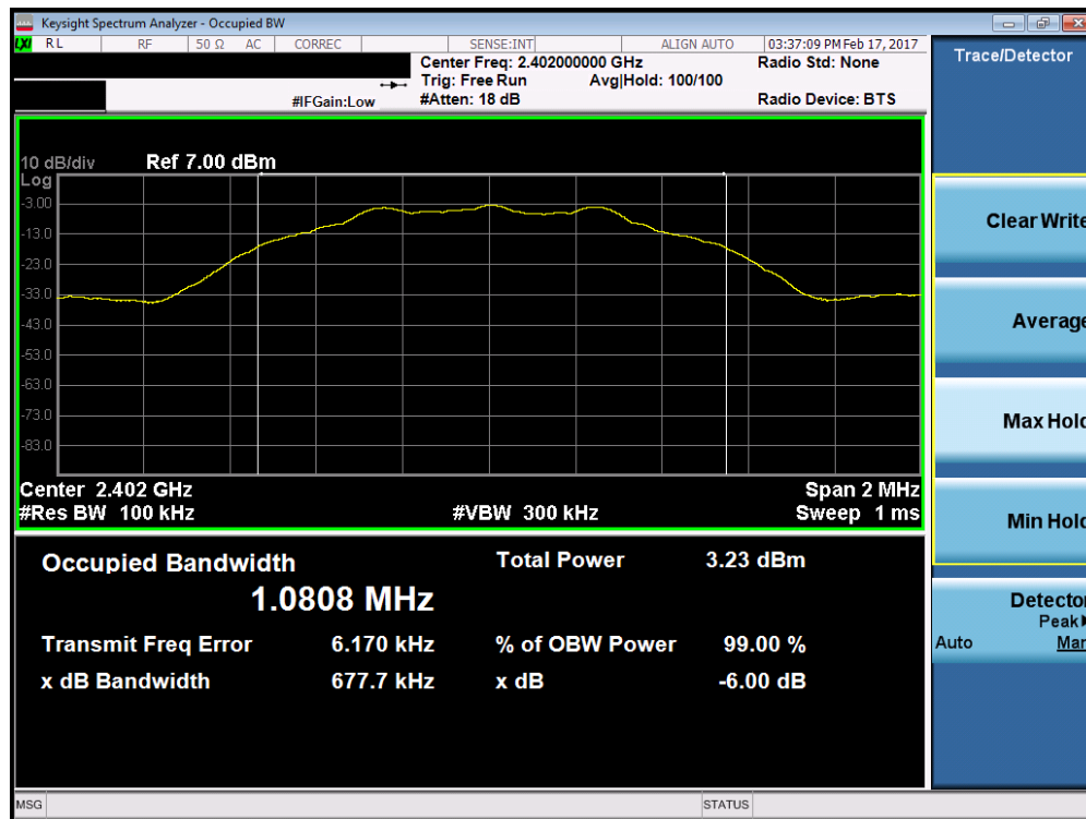
Plot 7-1. 6dB Bandwidth Plot (Bluetooth (LE) – Ch. 0)
