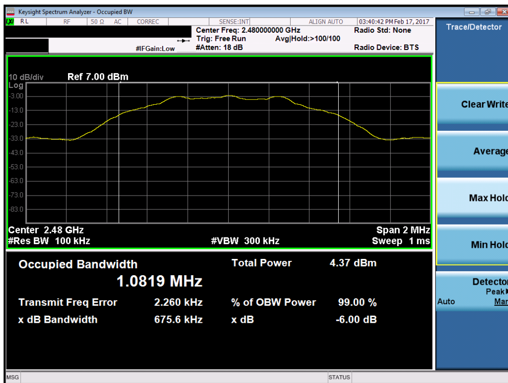
Plot 7-3. 6dB Bandwidth Plot (Bluetooth (LE) – Ch. 39)
