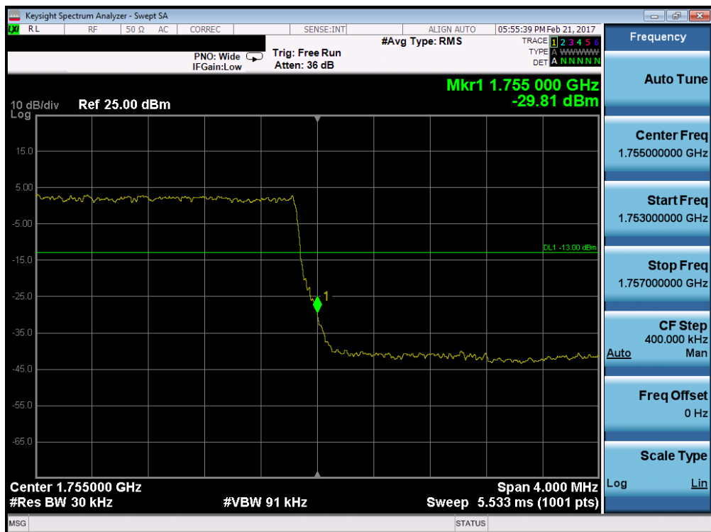
Plot 7-68. Upper Band Edge Plot (Band 4 – 3.0MHz QPSK – RB Size 15)
