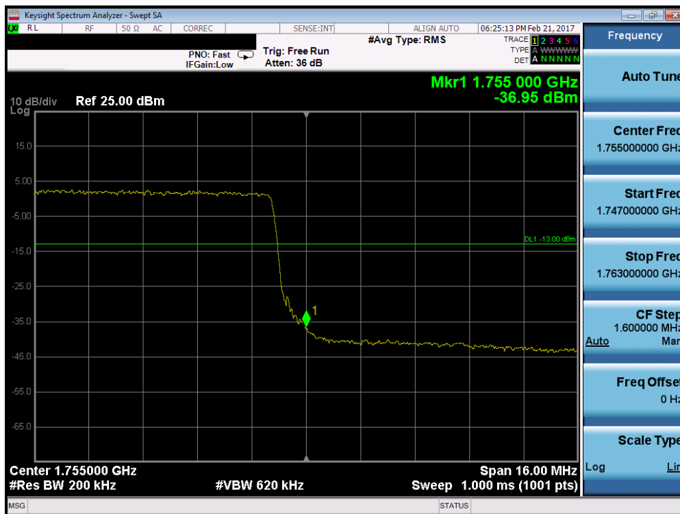
Plot 7-84. Upper Band Edge Plot (Band 4 – 20.0MHz QPSK – RB Size 100)
