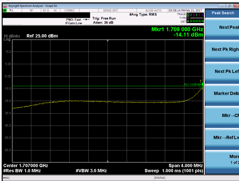
Plot 7-71. Lower Extended Band Edge Plot (Band 4 - 5.0MHz QPSK - RB Size 25)
