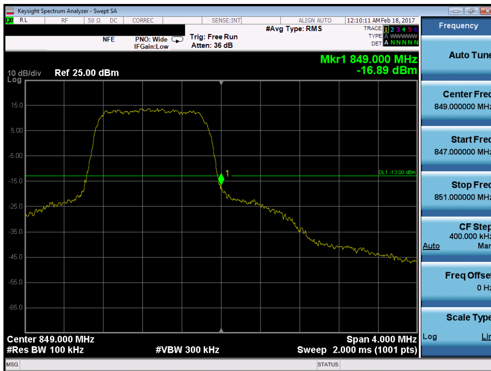
Plot 7-55. Upper Band Edge Plot (Band 5 – 1.4MHz QPSK – RB Size 6)
