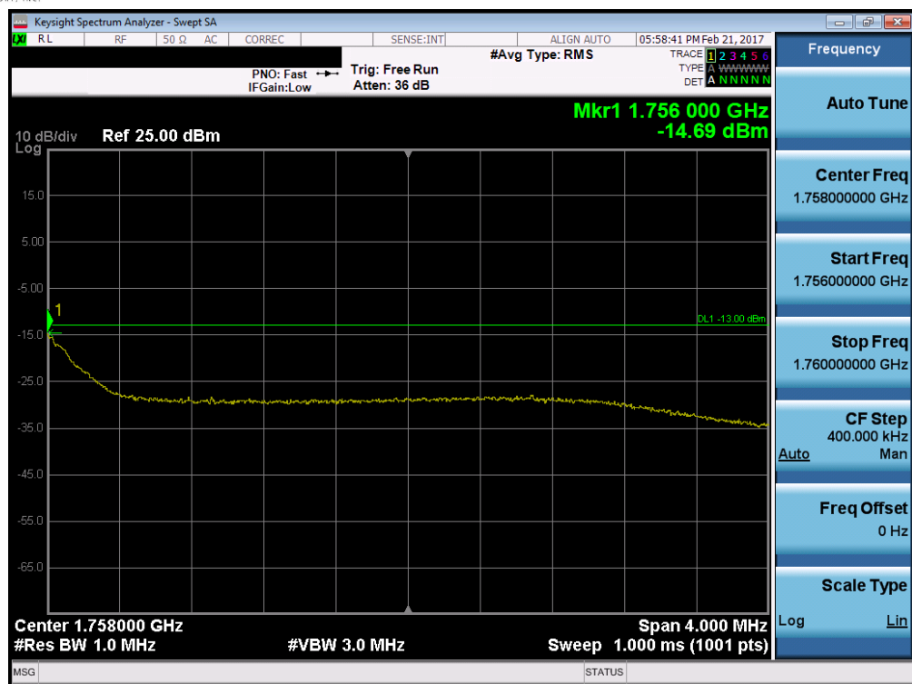
Plot 7-73. Upper Extended Band Edge Plot (Band 4 – 5.0MHz QPSK – RB Size 25)
