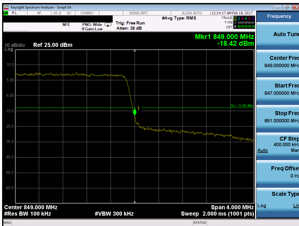
Plot 7-57. Upper Band Edge Plot (Band 5 – 3.0MHz QPSK – RB Size 15)
