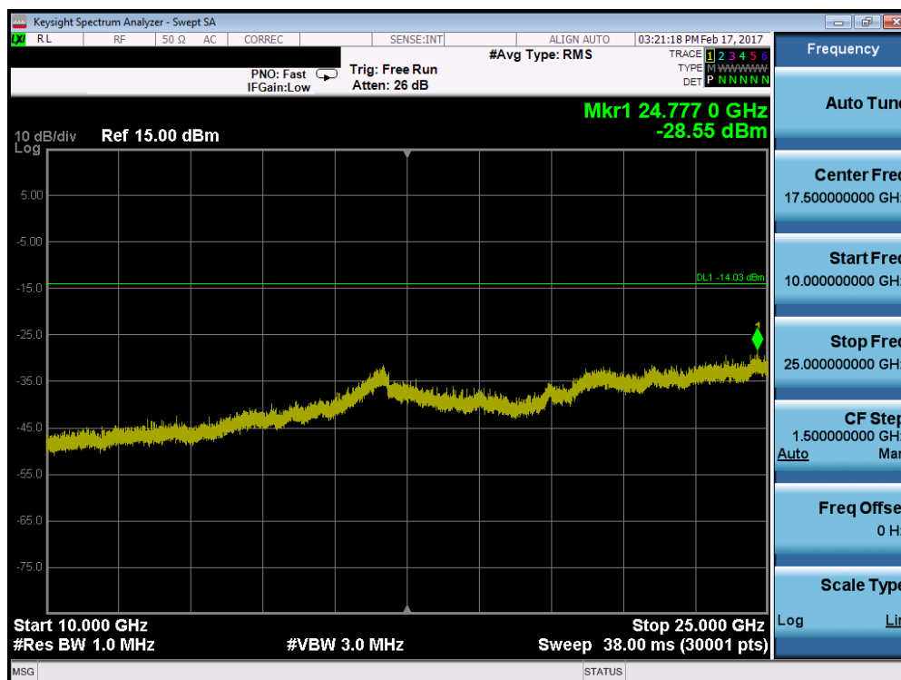
Plot 7-37. Conducted Spurious Plot (Bluetooth, 3Mbps – Ch. 0)
