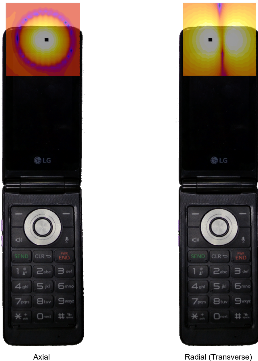
Figure 14-3 T-Coil Scan Overlay Magnetic Field Distributions
