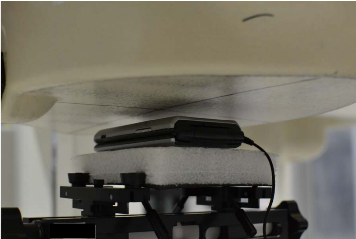
SAR Test Setup Photo 7 – Back Side with Headphones at 10 mm
