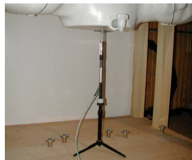
Figure 12-2 System Verification Setup Photo
