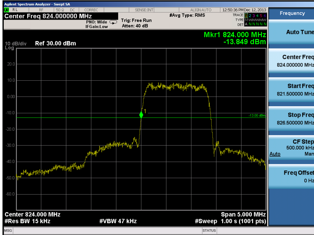
Plot 6-15. Band Edge Plot (Cellular CDMA Mode – Ch. 1013)
