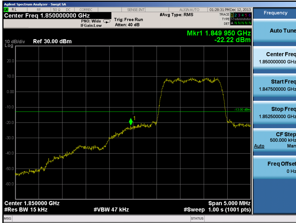
Plot 6-17. Band Edge Plot (PCS CDMA Mode – Ch. 25)
