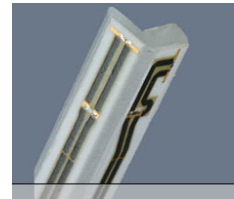
Figure 4-1 E-field Free-space Probe
