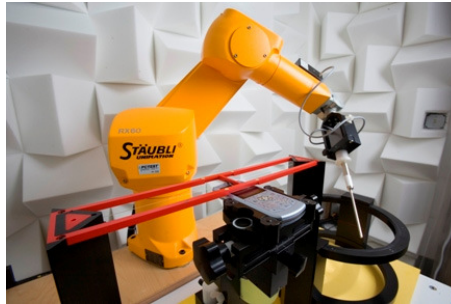
Figure 4-3 SPEAG Robotic System
