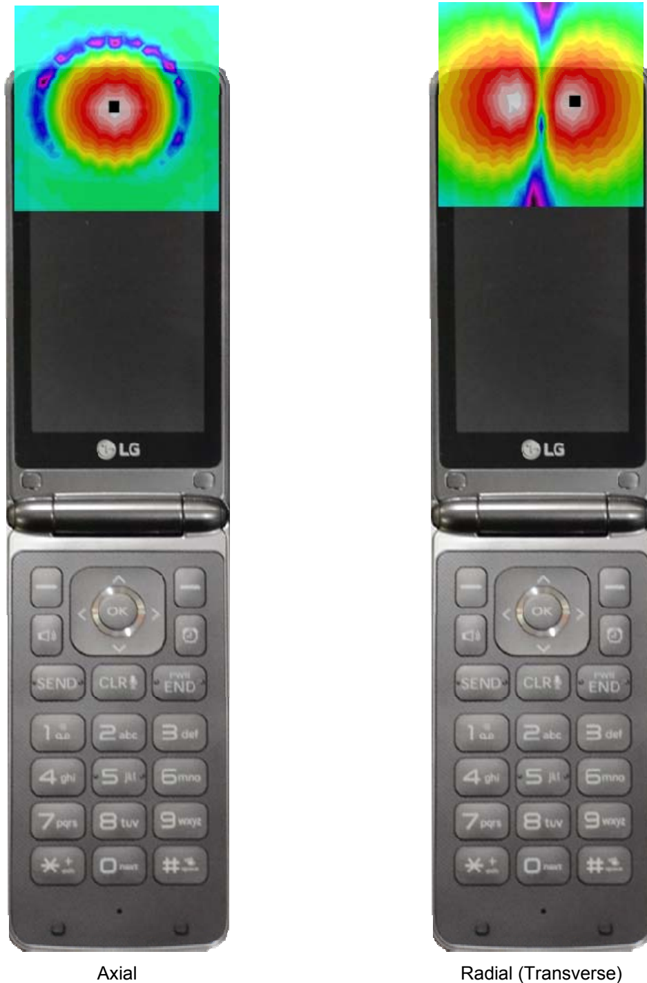
Figure 12-3 T-Coil Scan Overlay Magnetic Field Distributions
