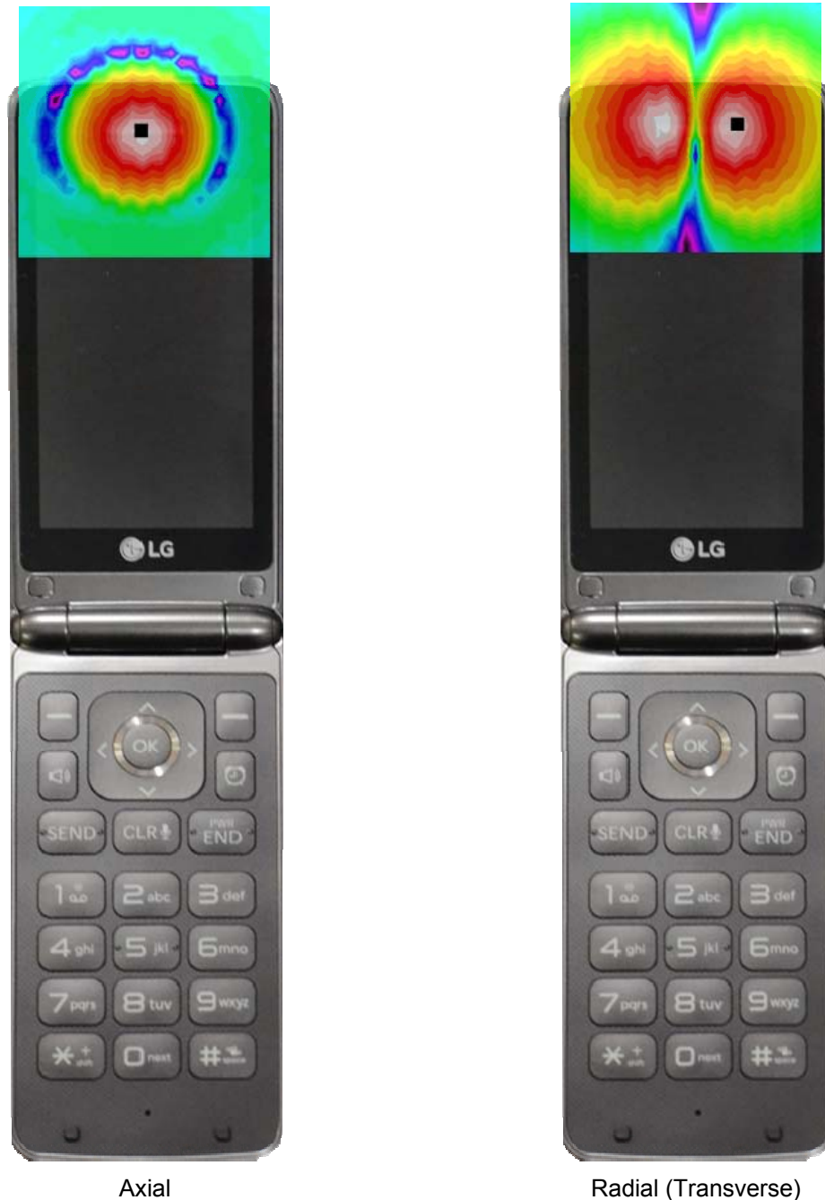
Figure 13-3 T-Coil Scan Overlay Magnetic Field Distributions
