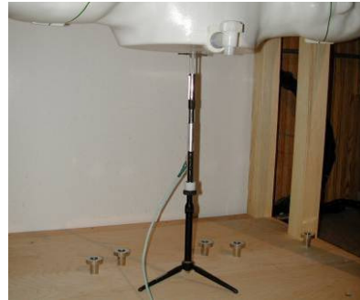
Figure 10-2 System Verification Setup Photo
