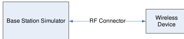
Figure 9-2 Power Measurement Setup
