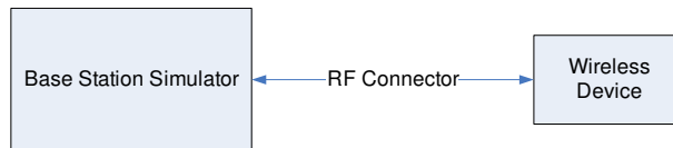
Figure 9-3 Power Measurement Setup
