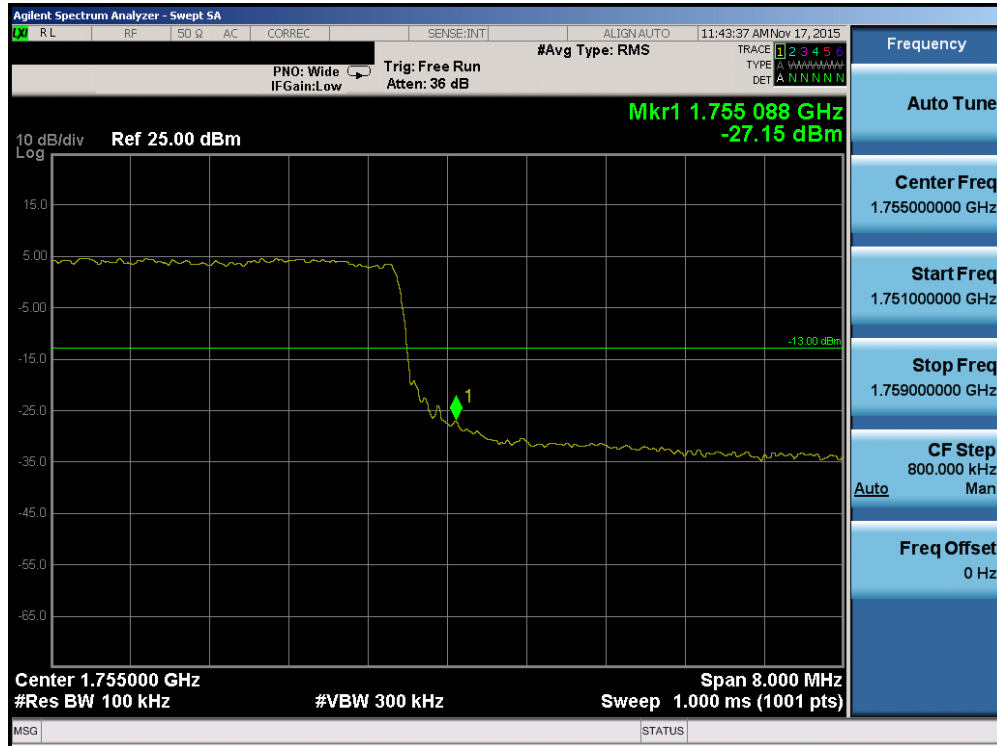
Plot 7-112. Upper Band Edge Plot (Band 4 – 10.0MHz QPSK – RB Size 50)
