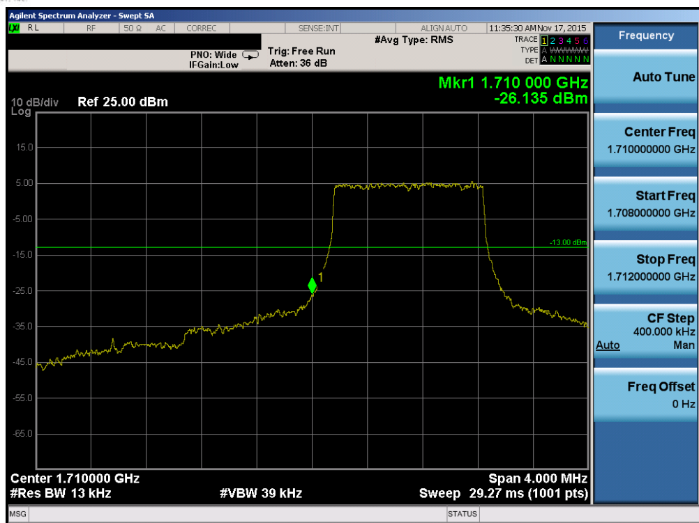
Plot 7-98. Lower Band Edge Plot (Band 4 – 1.4MHz QPSK – RB Size 6)
