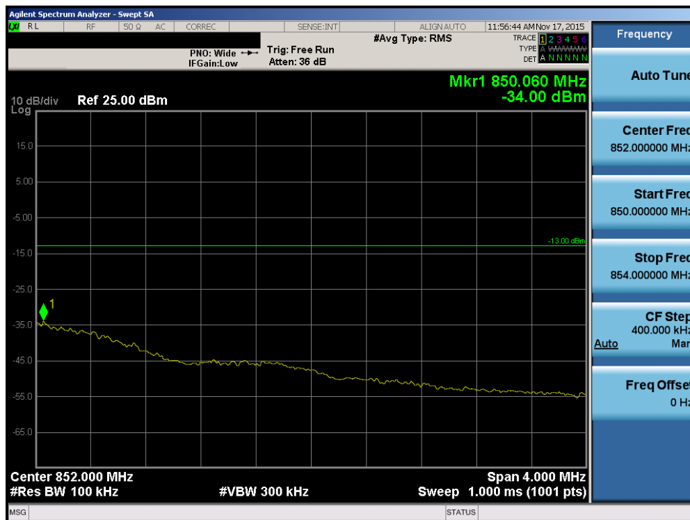
Plot 7-87. Upper Extended Band Edge Plot (Band 5 – 1.4MHz QPSK – RB Size 6)
