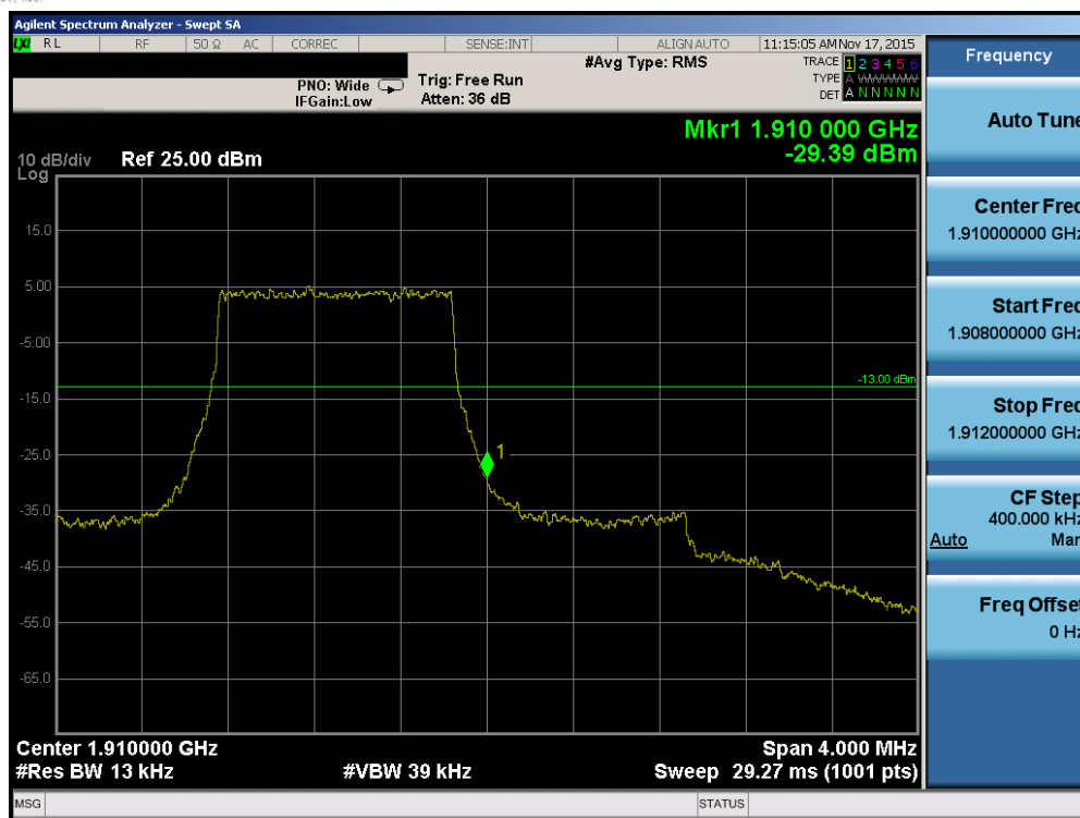
Plot 7-124. Upper Band Edge Plot (Band 2 – 1.4MHz QPSK – RB Size 6)
