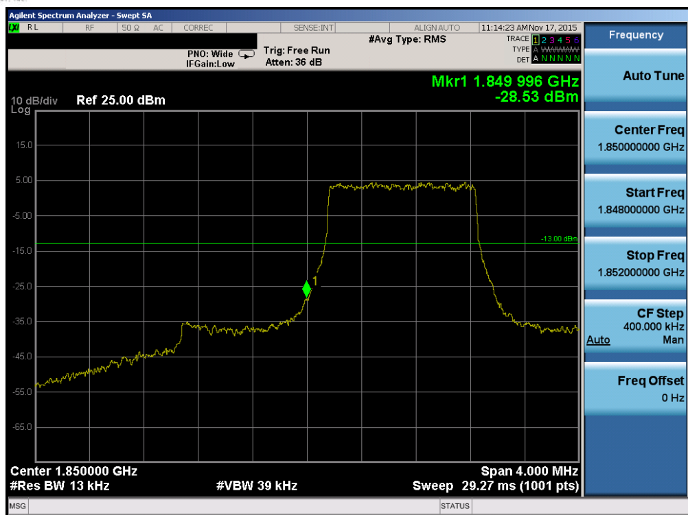
Plot 7-122. Lower Band Edge Plot (Band 2 – 1.4MHz QPSK – RB Size 6)
