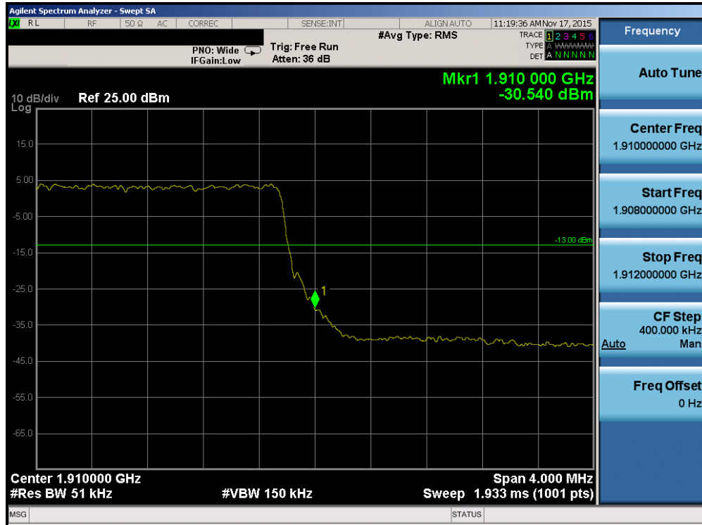
Plot 7-132. Upper Band Edge Plot (Band 2 – 5.0MHz QPSK – RB Size 25)
