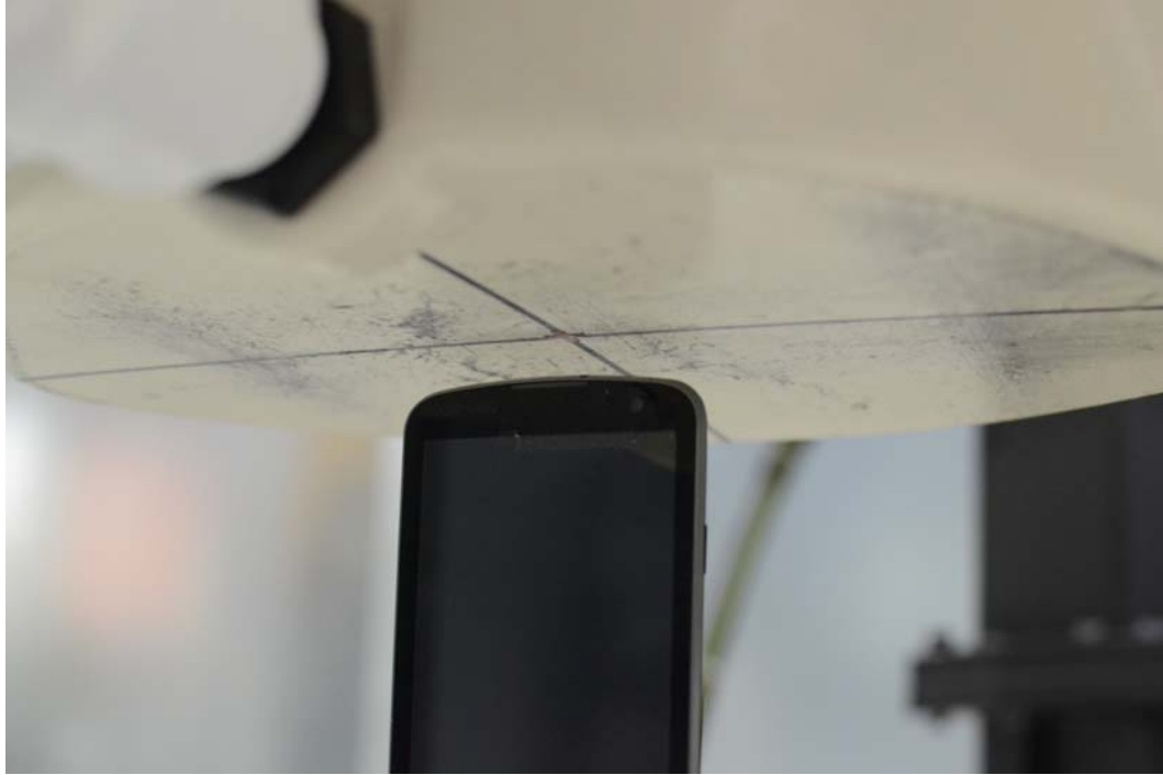
SAR Test Setup Photo 7: Top Edge 1.0 cm
