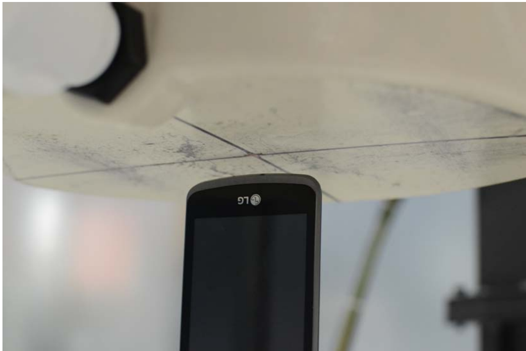
SAR Test Setup Photo 8: Bottom Edge 1.0 cm
