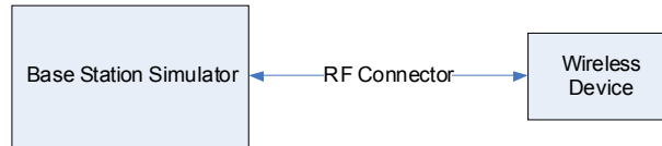
Figure 9-3 Power Measurement Setup
