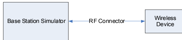
Figure 9-2 Power Measurement Setup
