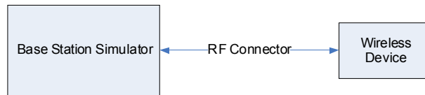
Figure 9-3 Power Measurement Setup
