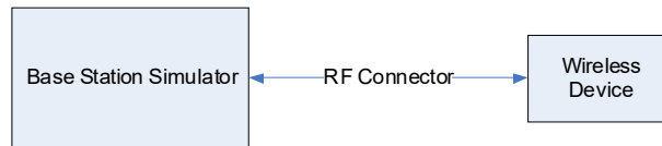
Figure 9-3 Power Measurement Setup
