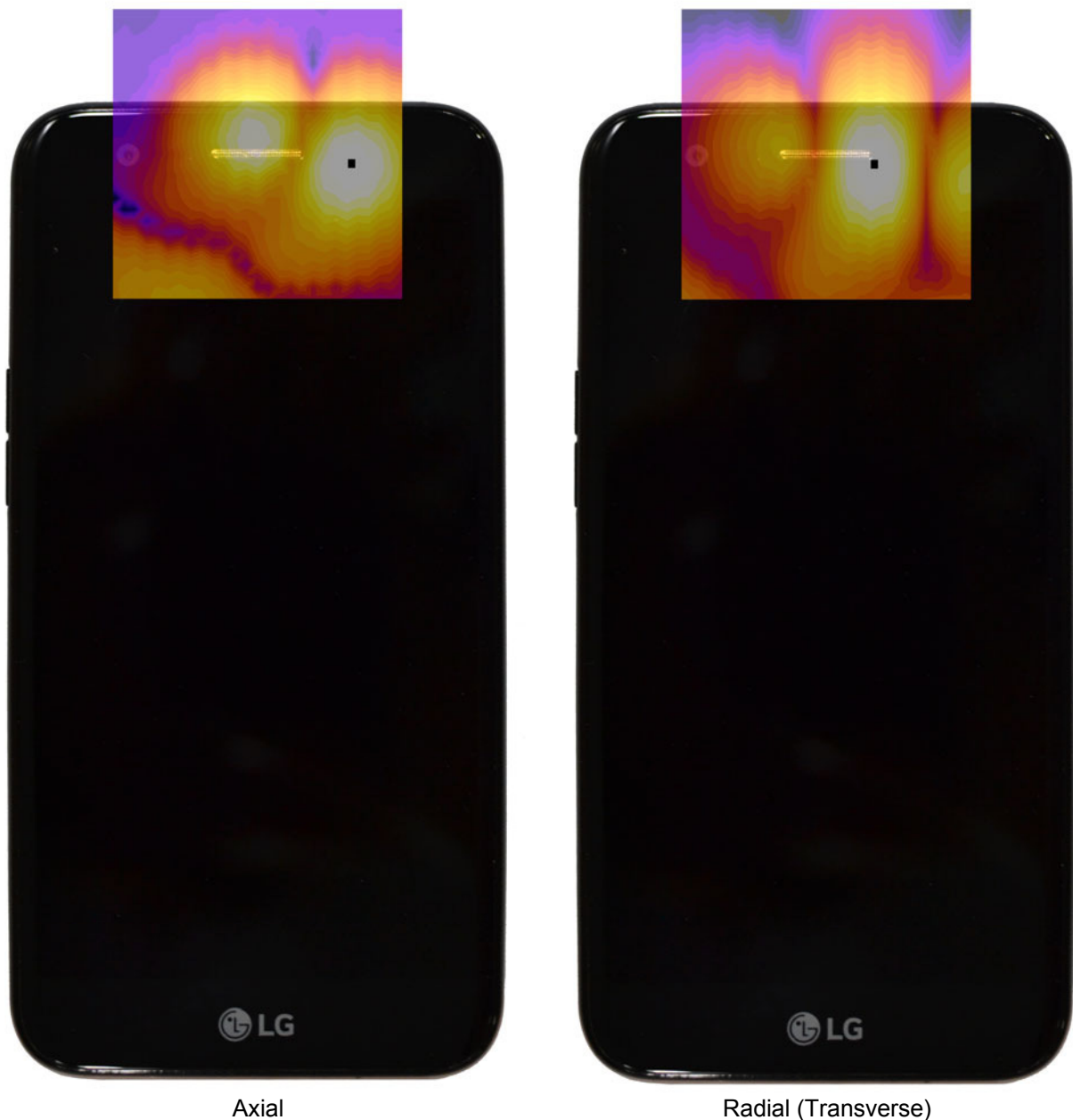
Figure 14-3 T-Coil Scan Overlay Magnetic Field Distributions
