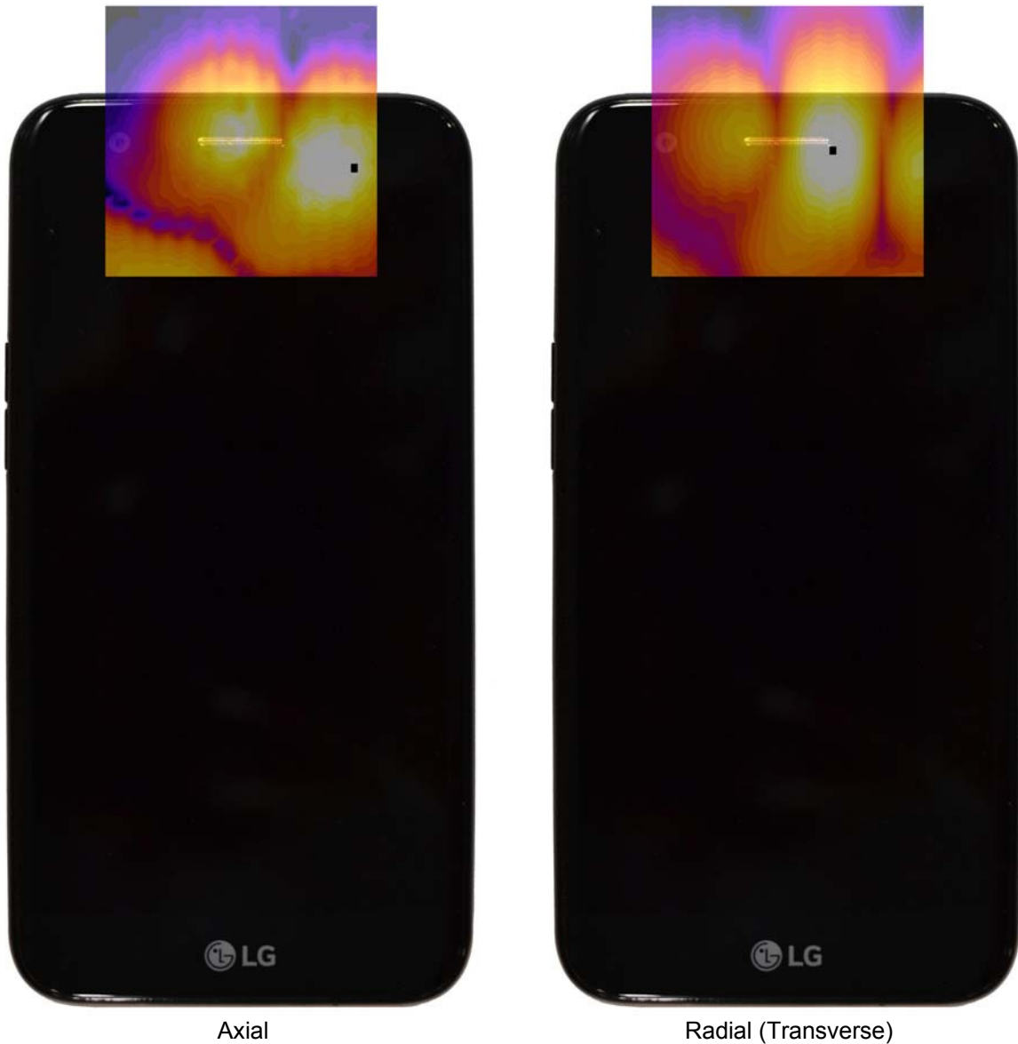
Figure 14-3 T-Coil Scan Overlay Magnetic Field Distributions
