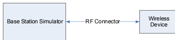
Figure 9-3 Power Measurement Setup
