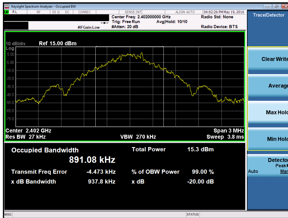
Plot 7-1. 20dB Bandwidth Plot (Bluetooth, 1Mbps – Ch. 0)
