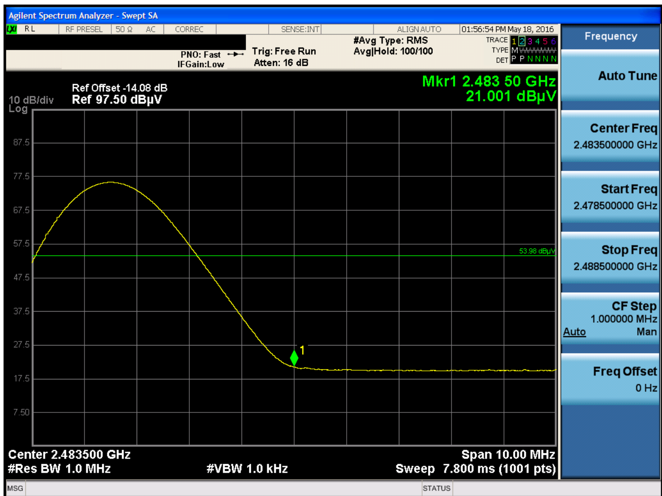
Plot 7-50. Radiated Restricted Upper Band Edge Measurement (Average)
