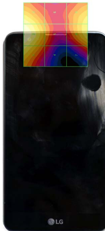
Figure 17-4 E-Field WD Scan overlay
