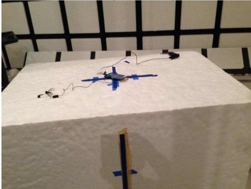
RADIATED FRONT PHOTO (BELOW 1 GHz)
