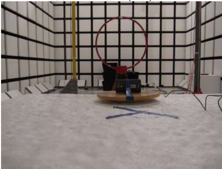
RADIATED EMISSIONS BELOW 30MHz (BACK)
