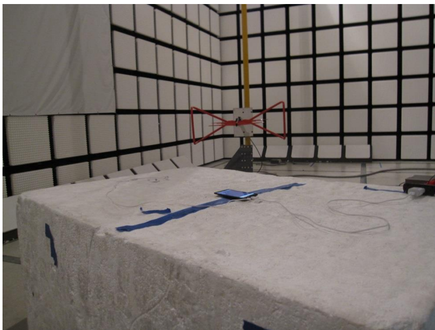
RADIATED BACK PHOTO (BELOW 1 GHz)
