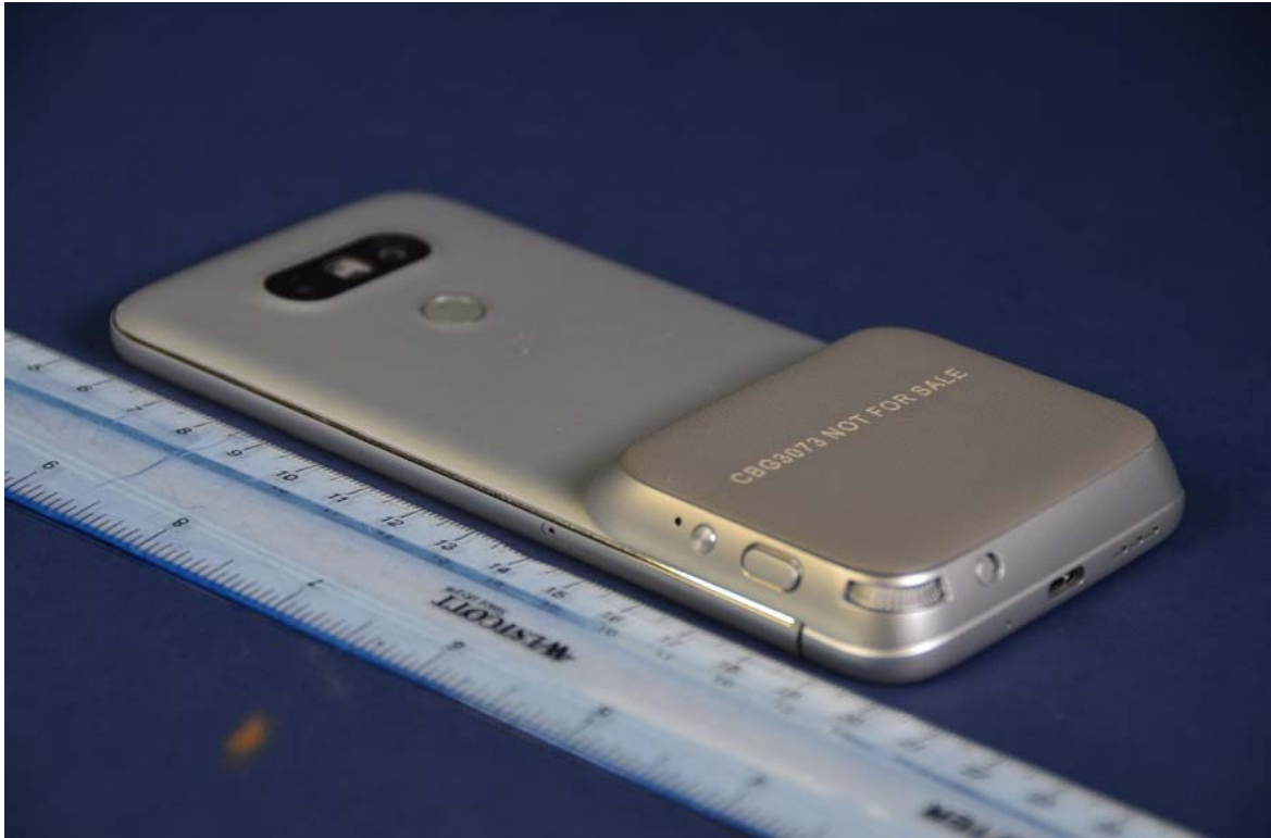
Camera Module Installed
