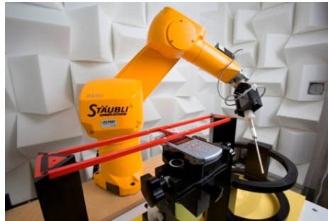
Figure 5-3 SPEAG Robotic System
