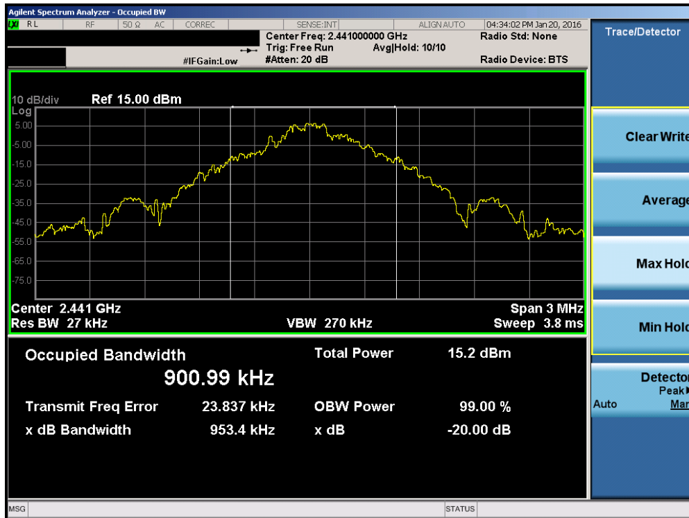
Plot 7-2. 20dB Bandwidth Plot (Bluetooth, 1Mbps – Ch. 39)
